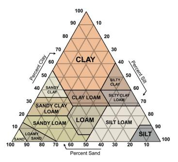
Fig. 6.1 USDA textural triangle for soil textural class determination
